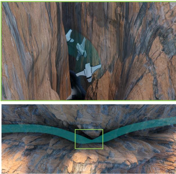
Fig. 15. Owing to the precise collision representation in the SVSDF, the spacecraft efficiently plans continuous, collision-free trajectories in extremely confined canyon spaces. This performance exceeds that of planning methods that rely on discrete collision evaluation.
